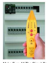
Make Sure All The Circuit Breakers Are On Now, for example, start scanning from the top left row, then go down etc..., But you can scan the breakers in any order. While you are scanning, observe the bar-graph and listen to the buzzer.
