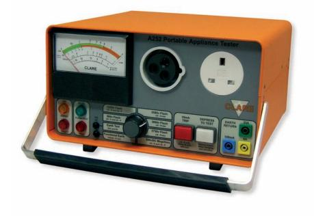
This versatile portable test set is easy to operate and carries out effective electrical safety testing of office equipment, power tools and appliances.
